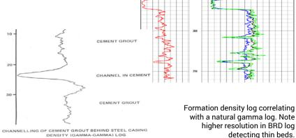
with a natural gamma log. Note higher resolution in BRD loa detecting thin beds.
